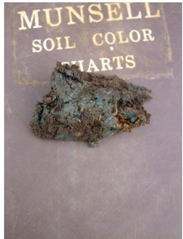
The picture on the left shows the Klukkufell profile. The picture on the right shows a blue redox color ( \text{Fe}^{2+} ) that was found on the 2Bw horizon.
