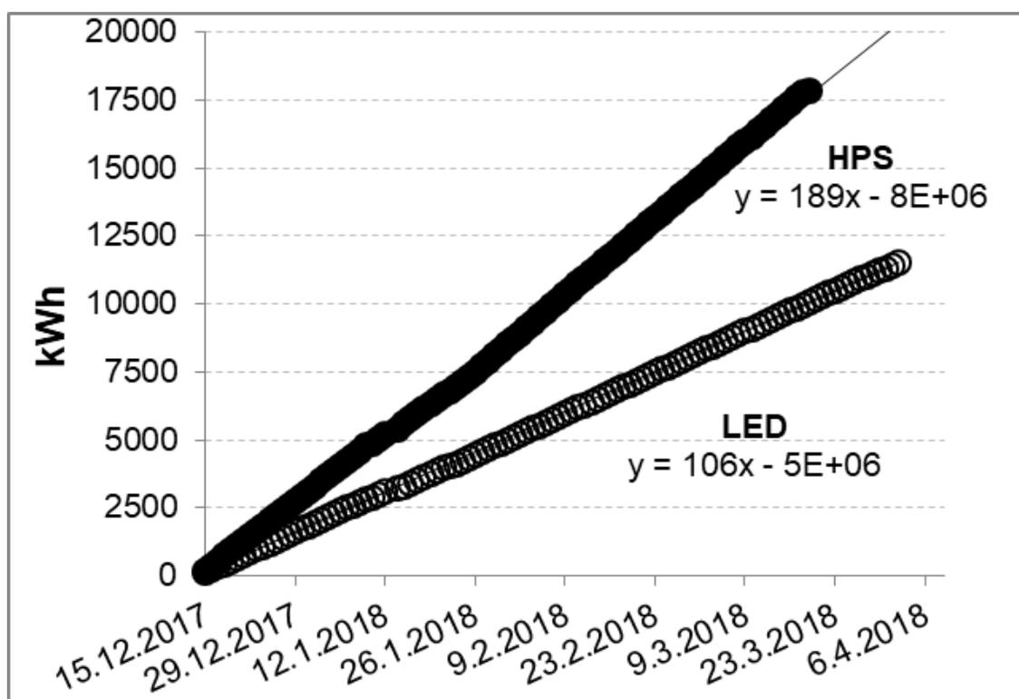
Fig. 25: Used kWh in the different chambers.
